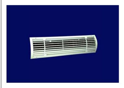
It is suitable for oval ducts and round ducts and fitted flush with the duct without using a duct collar. The grills are fitted with extruded aluminium powder coated collar damper to control the quantity of supply air.
