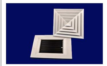
A view of the supply air diffusres of neck size 375 x 375 mm and having an outer size of 595 x595 mm fitted with extruded aluminium powder coated collar damper. The centre core of the diffuser ican be removed without any tools and it is spring loaded.
